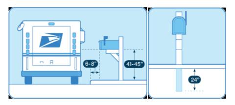
If you're mounting a curbside mailbox on a post near the street, the support should be secure and safe. The best supports are designed to bend or fall away if a car hits them.
