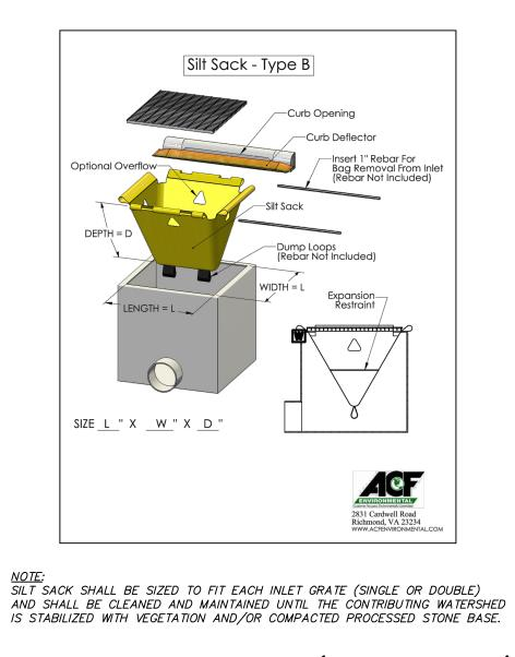
INLET PROTECTION (SILT SACK) NOT TO SCALE
