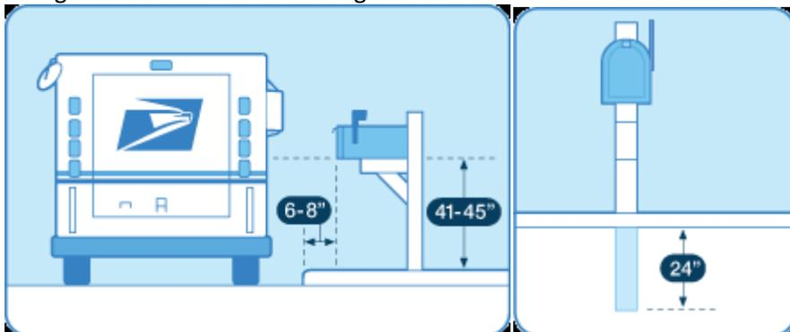
For curbside mailboxes on a post near the street, the support should be secure and safe. The best supports are designed to bend or fall away if a car hits them.
